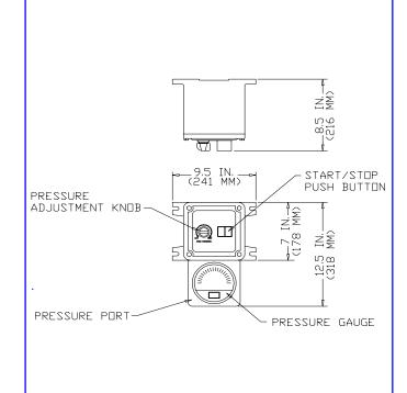
Figure 5: Remote Control Box (PBX 10-01)
