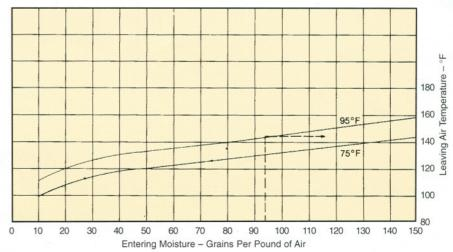
LEAVING AIR TEMPERATURE - °F FOR INLET TEMPERATURE BELOW 75°F, SUBTRACT TEMPERATURE DIFFERENCE FROM OUTLET TEMPERATURE
