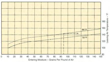
LEAVING AIR TEMPERATURE - °F FOR INLET TEMPERATURE BELOW 75°F, SUBTRACT TEMPERATURE DIFFERENCE FROM OUTLET TEMPERATURE
